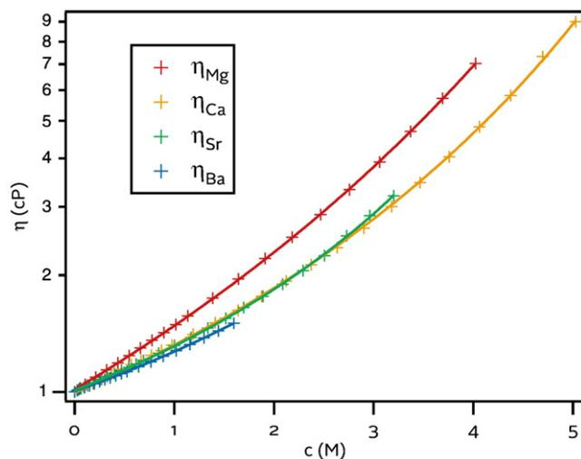
Fig. 5. The macroscopic shear viscosity of aqueous solutions of some divalent cations [88]. In all cases, the anion is chloride. Notice that the viscosity scale is logarithmic.
