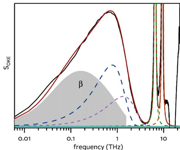
**Fig. 8.** OKE data for carbon tetrachloride at 25 °C transformed to the frequency domain and deconvoluted. Data (black solid line), fit (red solid line), and a decomposition of the fit into a cage-rattling  $\beta$ -relaxation mode (stretched-exponential decay with  $\beta = 0.6$ ), two anti-symmetrized Gaussian bands, and two harmonic oscillators corresponding to intramolecular vibrational modes.
