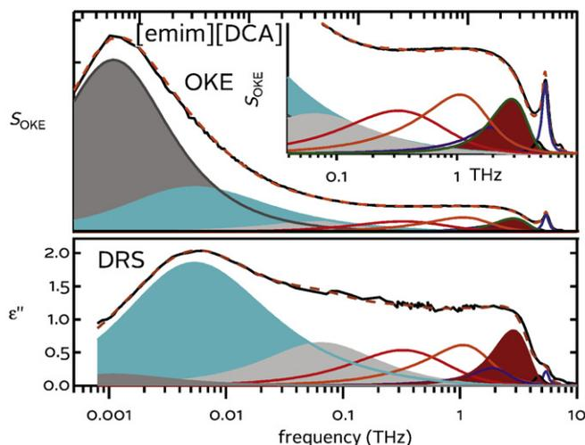
Fig. 3. An OKE spectrum (top) and dielectric spectrum (bottom) of the room-temperature ionic liquid 1-ethyl-3-methylimidazolium dicyanamide (emim DCA). Comparison of the two spectra allows one to identify a sub- $\alpha$  relaxation peak due to mesoscopic structure that is only clearly visible in the OKE spectrum. [16].
