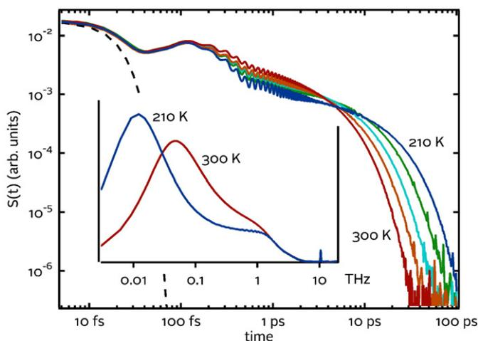
Fig. 2. OKE measurements on trans-1,2-dichloroethene in the time-domain showing, on logarithmic axes, five sets of data measured at 210, 230, 250, 270, and 300 K. The instrument response (autocorrelation) is also shown (dashed). The inset shows the signals at the lowest and highest temperatures in the frequency domain. [72].
