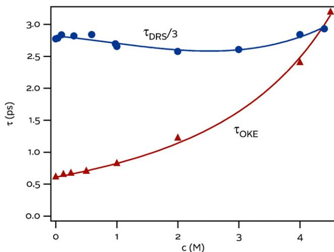
Fig. 4. Relaxation times of aqueous solutions of MgCl<sub>2</sub> at 25 °C obtained using DRS (●) and OKE spectroscopy (▲). The DRS relaxation time has been divided by a factor of 3. The DRS relaxation is associated with rotational motion while the OKE relaxation is associated with translational motions [70].
