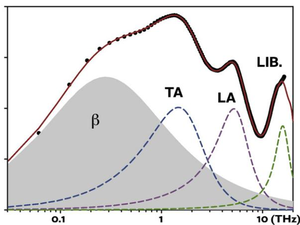
**Fig. 7.** OKE data for neat water at 25 °C transformed to the frequency domain and deconvoluted. Data (dots), fit (red solid line), and a decomposition of the fit into a cage-rattling  $\beta$ -relaxation mode, two damped harmonic oscillators (corresponding to hydrogen-bond bend and stretch modes), and a harmonic oscillator representing the onset of the librational band [70,71].
