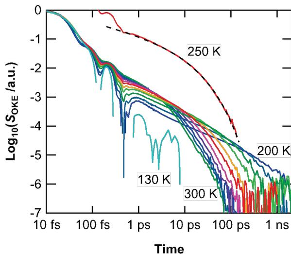
**Figure 4** For the eutectic solution of LiCl in water, OKE spectroscopy allows the measurement of the dynamics over around five orders of magnitude (in time and amplitude) from 300 K to 200 K and in the glassy state at 130 K. The 250 K signal is also shown vertically offset with the (stretched exponential) fit (dashed curve) showing the quality of fit over four orders of magnitude in amplitude.
