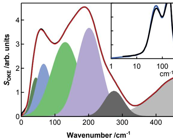
**Figure 3** The reduced Raman (OKE) spectrum (linear frequency scale) for the eutectic solution of LiCl at 130 K (black) can be fit accurately by the sum of six Gaussian functions (red). Inset is detail (on a log frequency scale) showing the anomalous mode below  $20\text{ cm}^{-1}$  with the almost identical spectrum of LiCl in  $\text{D}_2\text{O}$  (blue). For details and fit parameters see (Appendix A).
