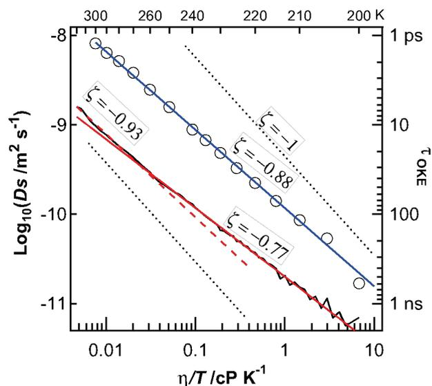
**Figure 6** Both OKE (circles) and NMR (black line) time constants show fractional Stokes-Einstein behaviour when plotted against viscosity. However, while the OKE data can be fitted by a constant exponent of 0.88, the NMR data break at around 250 K. Normal Stokes-Einstein behaviour is indicated by the dotted lines.
