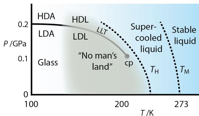
**Figure 1** The phase diagram proposed by Mishima and Stanley<sup>4</sup> for the non-crystalline states of water shows the putative second critical point **cp** that lies in the experimentally inaccessible region below the homogeneous nucleation temperature  $T_H$ . The liquid-liquid transition associated with this point arises from the observed transition between the high and low density amorphous phases.
