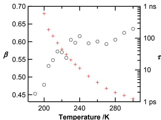
**Figure 5** The parameters for the fit of the stretched exponential to the OKE data for the eutectic solution of LiCl in water over the range of temperature from 300 K to 190 K. The time constant  $\tau$  (crosses) shows no sharp discontinuity but here the dynamic crossover is evident from the sudden increase in broadening through the stretching parameter  $\beta$  (circles) at 230 – 240 K.
